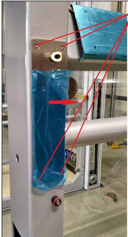
1. Unscrew 4 fixation bolts and take the lock out
