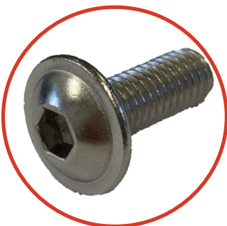
VIS 6 PANS TCB EMBASE M6x16 inox PR002698
